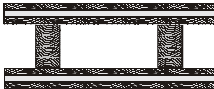
Cellular box girder cross section, e.g.: CLT, 3-l + GLT (GL24 to GL36) + CLT 3-l
